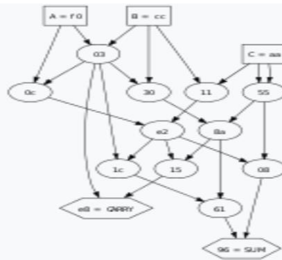
Fig 2.2 Nor full adder
